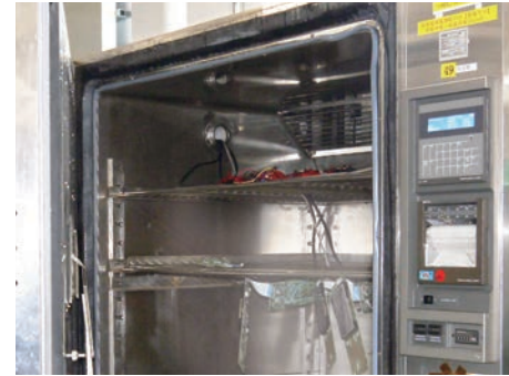
Circuit board stress test At temperature of -40°F to +185°C, relative humidity of 85%.
