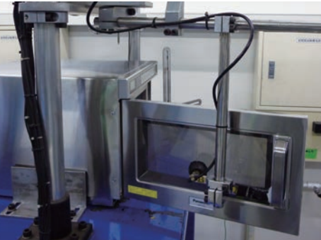
Door endurance test Panasonic puts their high-quality microwave ovens through over 400,000 door open-close tests before they get delivered to customers.
