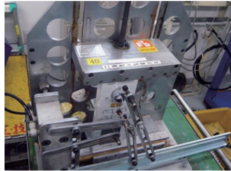
Control panel endurance test Operation of touch pads 200,000 times
