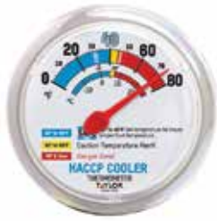
5636 6" Bi-Metal Thermometer HACCP Cooler/Freezer
